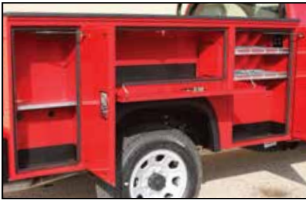
Durabed Liner in Loadspace and Compartment Floors
