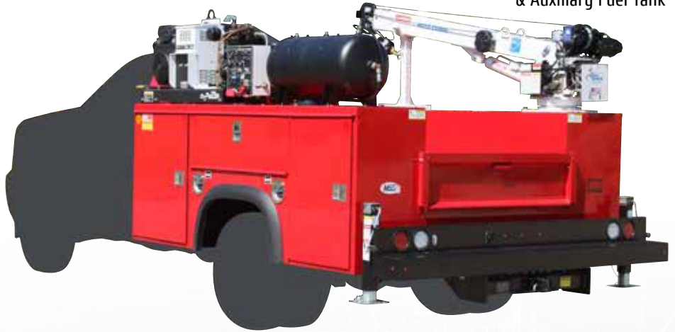
Crane, Air Compressor, Engine & Auxillary Fuel Tank
