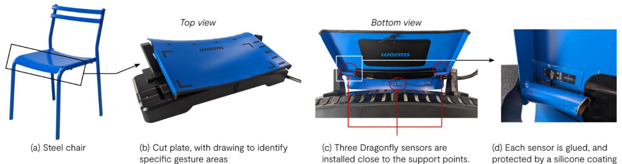
Figure 1: Transforming a basic steel chair into a tactile interface using three Dragonfly® strain sensors.
