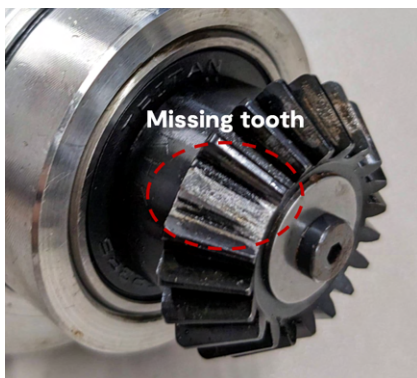
Gearbox with 20 teeth rotating at 1Hz .
