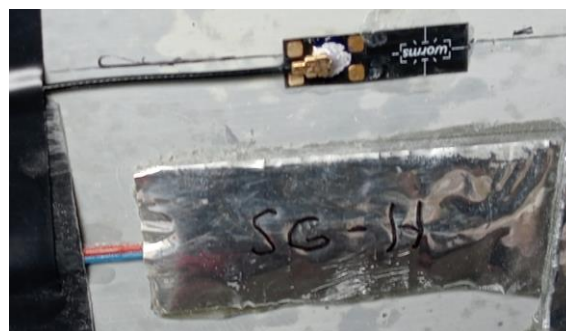
Figure 4: Dragonfly sensor before protective layer installation
