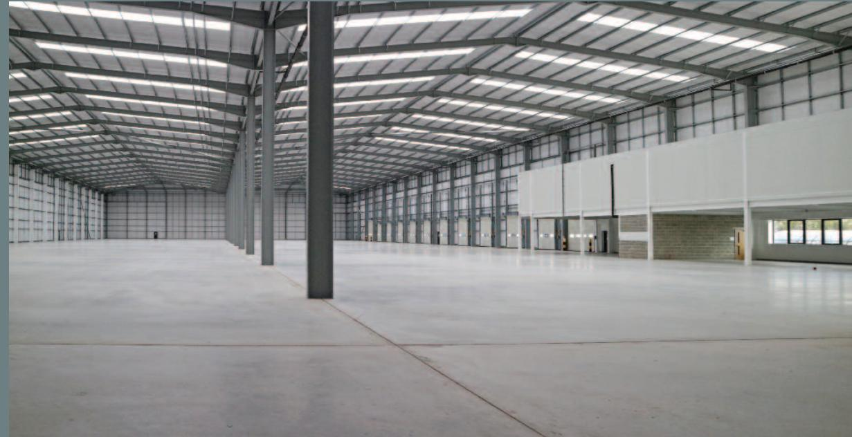
The property is a distribution warehouse unit constructed on a steel portal frame under a metal sheet roof. The warehouse has a concrete floor, 3 phase power, mains gas and a haunch height of 12 metres. Loading access is via 10 dock level loading doors and 2 ground level loading doors. The unit also benefits from ancillary office accommodation, WC facilities and a self contained secure yard area to the front elevation.
