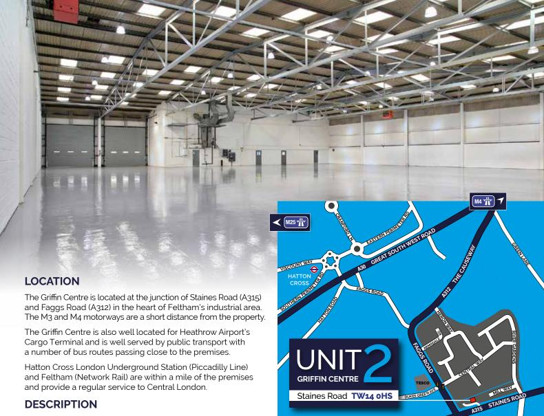
Unit 2 is of steel truss frame construction and two storey office accommodation with two loading doors. Internally the warehouse benefits from 7.4m eaves and provides clear span warehouse accommodation.
