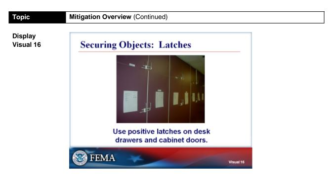
Secure loose drawers and cabinet doors with positive latches. Positive latches prevent the drawers and cabinets from swinging open and can keep the contents from spilling out.
