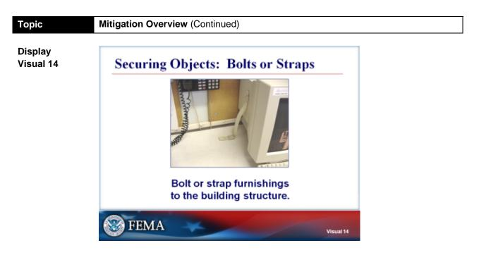
Secure objects by bolting or strapping furnishings to the building structure.
