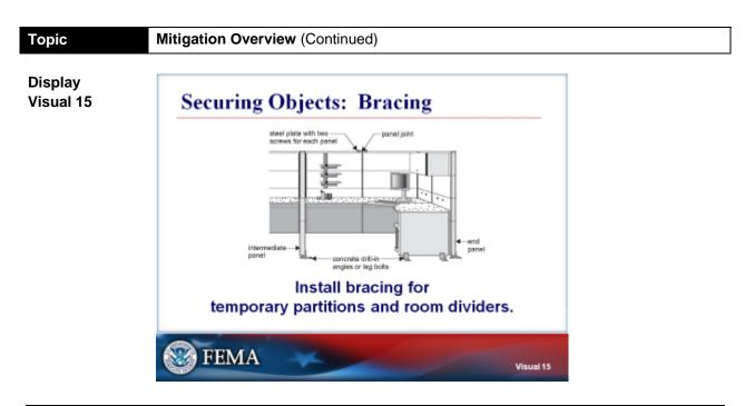
Another means of securing loose objects is to install bracing. For instance, ensure that any temporary partitions and room dividers are secured.
