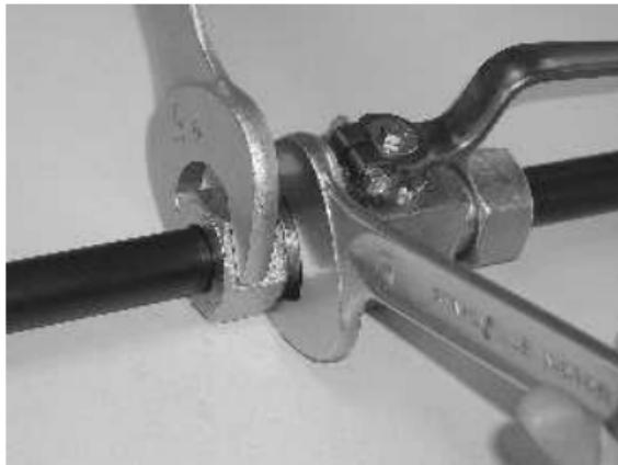
In the case of ball valves with weld-type connections, ensure that no weld particles get inside the valve during installation. Weld deposits must be removed without fail. It is also important to ensure that the inside of the ball valve does not exceed the permissible operating temperature. Exceeding the operating temperature can result in damage to the seals.
