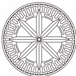
Reamer with bigger holes for more pulp content
