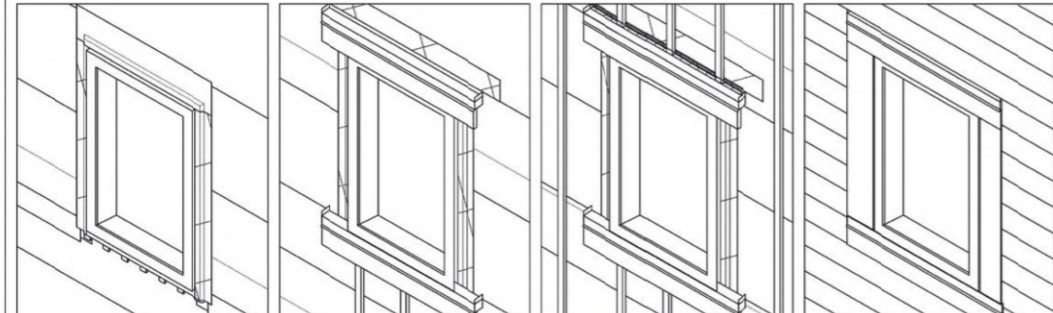
9. APPLY S.A.M. OVER JAMB FLANGES & MIN. 2" ONTO B.P. LAP B.P. OVER RETAINING CLIP AND HEAD FLANGE. 10. INSTALL SUBTRIM OVER HEAD AND SILL FLANGES. INSTALL TRIM AND FLASHINGS WITH REQUIRED STRAPPING. INSTALL S.A.M. FROM SHEATHING ONTO HEAD FLASHING. 11. COMPLETE B.P., INSECT SCREEN, & VERTICAL STRAPPING. 12. INSTALL SUBTRIM OVER JAMB FLANGES. INSTALL WALL CLADDING. CAULK JOINT BETWEEN JAMB SUBTRIM & WINDOW FRAME AND SUBTRIM & CLADDING. INSTALL JAMB TRIM.
