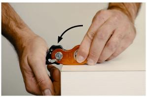
Use one hand to hold the device by the connection hole. With the other hand, rotate the cam outward and press down firmly with the palm. Finally, release the cam.
