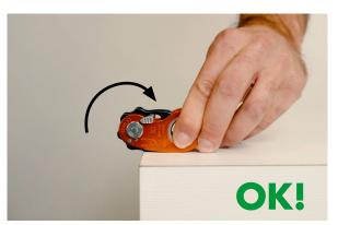
If the cam returns to its original position, it means that the product is not defective and can be used freely.
