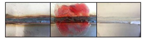
Once the reaction time has elapsed, wash thoroughly with cold and clean water if possible under pressure. The washing water must be tap and must not contain iron and chloride ions in concentration higher than 70 mg / L (conductivity  $\chi$ < 450  $\mu$ S).
