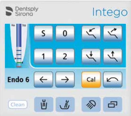
ApexLocator An ApexLocator can also be integrated into the EasyTouch to allow for permanent control of the working depth during endodontic treatment and a reduction of X-ray exposure.
