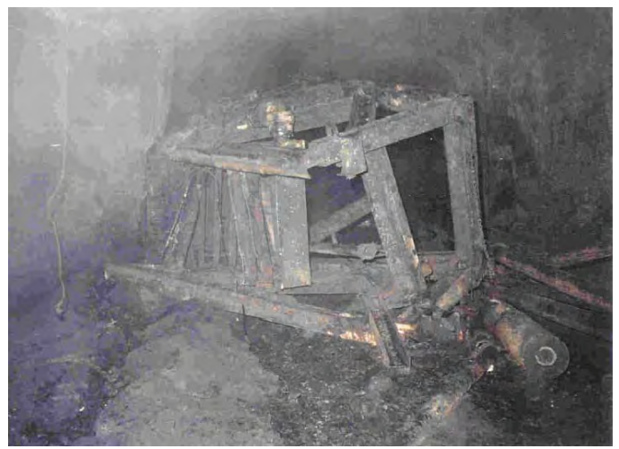
Figure 21.14D Photographs of roof falls, dislodged steel arches, and damaged equipment. Westray Mine Public Inquiry, Exhibit No. 59 (Richard, 1997).
