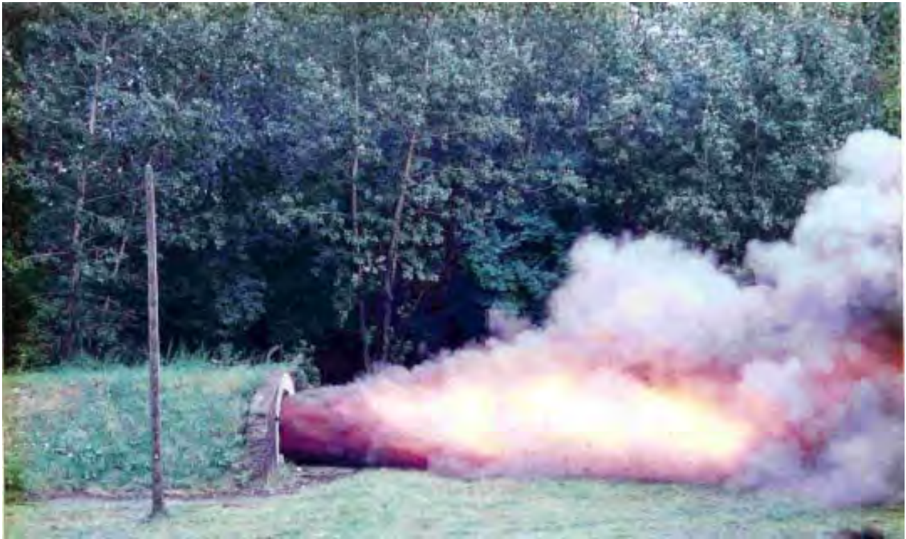
Figure 24.14B. The flame of a coal dust explosion emerging from a 2.5 m (8ft) high test gallery at the Barbara Mine, Poland
