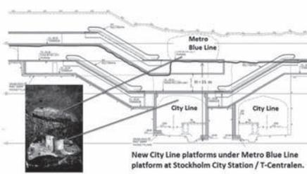
Figure 15. Excavating the 57, 200 m<sup>3</sup> City Line platform chambers directly under the metro.
