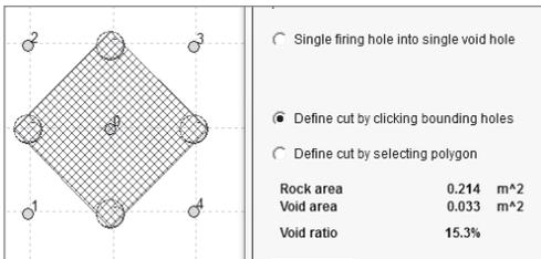
Figure 1. Burn cut showing meaningless void calculation.
