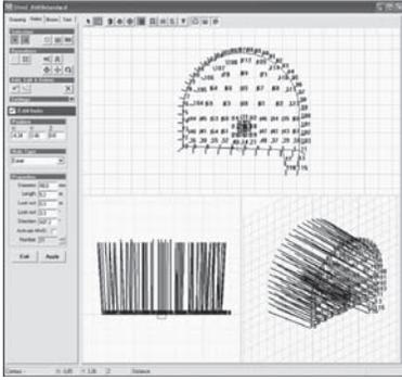
Figure 12. Design tool for drill plan generation.
