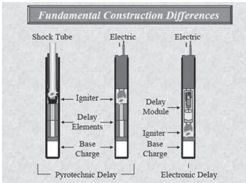
Figure 5. Construction of Electric, Shock-tube & Electronic Detonators © IME 2002.
