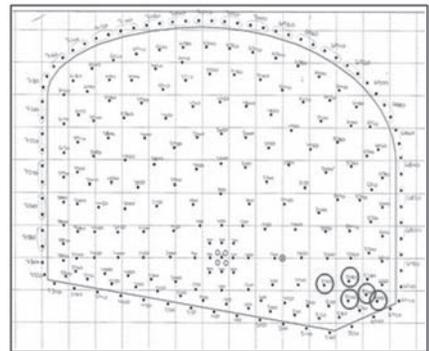
Figure 7. Correlating PPVs with shotholes the blast plan.
