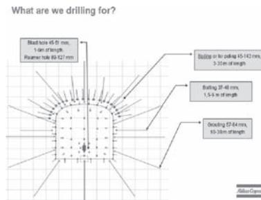
Figure 1. Drilling application.
