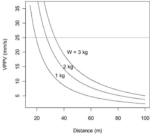
Figure 14. Vector peak particle velocity versus distance for a charge weight of 1, 2 and 3 kg. The plot is based on the 95% regression line for the combined data (Table 6). The AS 2187-2006 limit for human comfort for a component peak value is 25 mm/s (dashed line).
