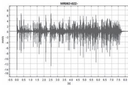
Figure 17. NCVIB: Example of blast vibration time history.
