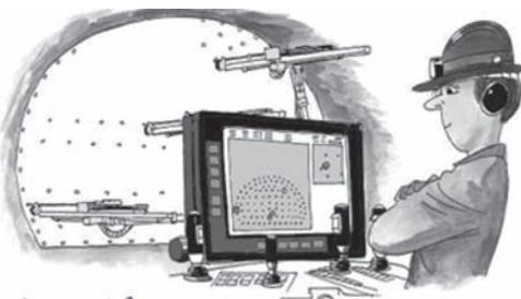
Figure 5. Automated collaring with ABC total.
