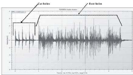
Figure 6. Vibration trace from a complete blast round.
