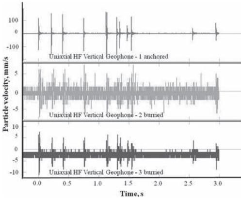
Figure 3. Signals obtained by different methods of coupling.
