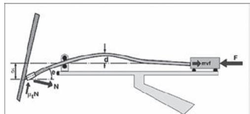
Figure 6. Drill hole deviation during drilling.
