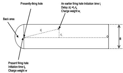
Figure 3. Path area where the earlier firing charges are accounted for screening the blast vibration from the presently-firing hole.
