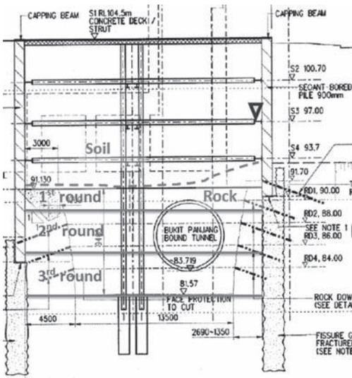
Figure 4. Section view of the shaft.
