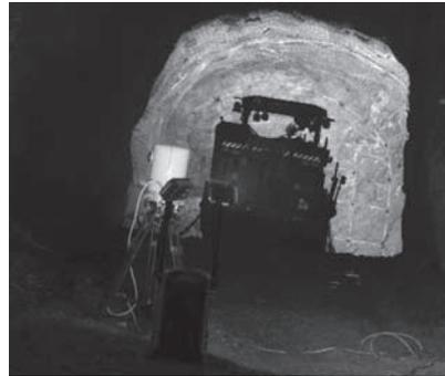
Figure 1. Laser scanning the wall of a tunnel (here the Callidus unit). Lighting is used for photographs and is not needed for acquiring the point cloud data alone.
