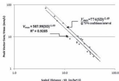
Figure 3. Vibration attenuation equation for the trial blasts.
