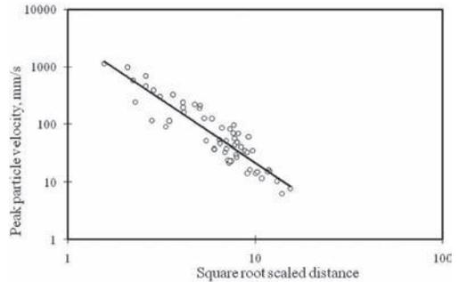
Figure 5. Peak particle velocity versus scaled distance.
