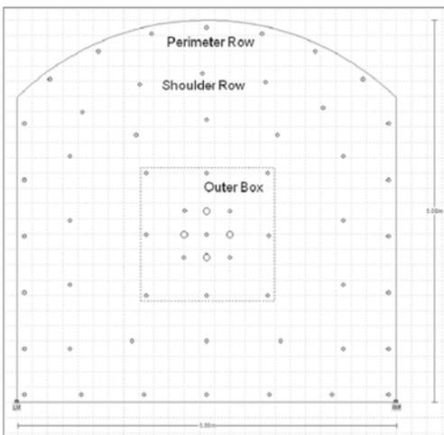
Figure 5. Face pattern showing areas of drilling.
