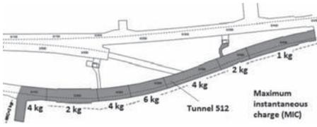
Figure 8. Instantaneous charge weight restrictions in tunnel 512.
