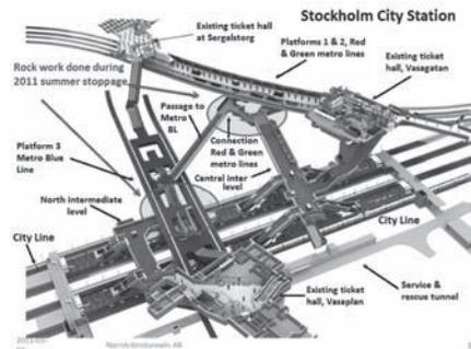
Figure 14. About 470 000 m<sup>3</sup> of rock was excavated to make space for Stockholm City Station, a multi-modal interchange.
