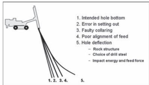
Figure 2. Factors that effects the drilling precision.
