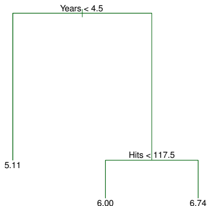
FIGURE 8.1. For the Hitters data, a regression tree for predicting the log salary of a baseball player, based on the number of years that he has played in the major leagues and the number of hits that he made in the previous year. At a given internal node, the label (of the form X_j < t_k ) indicates the left-hand branch emanating from that split, and the right-hand branch corresponds to X_j \geq t_k . For instance, the split at the top of the tree results in two large branches. The left-hand branch corresponds to Years < 4.5 , and the right-hand branch corresponds to Years >= 4.5 . The tree has two internal nodes and three terminal nodes, or leaves. The number in each leaf is the mean of the response for the observations that fall there.
