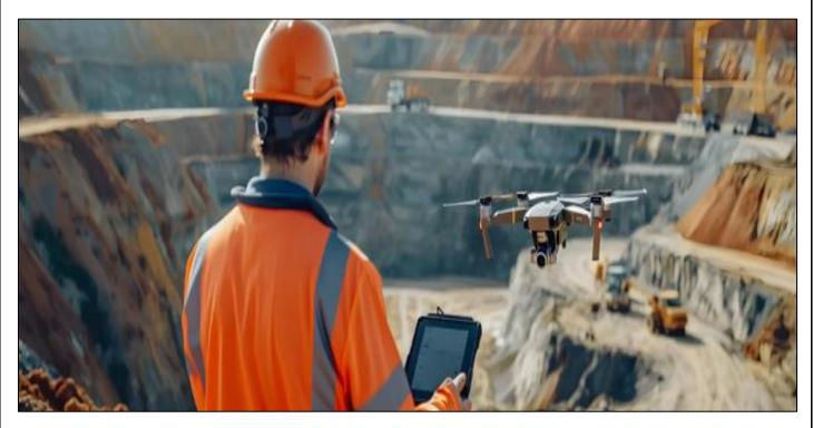
**Blast Optimization**: Drones can be utilized to map blast zones both before and after detonation, thereby furnishing valuable data for blast optimization and ensuring safety. Additionally, drone surveys can be employed to assess postblast fragmentation and strategically plan subsequent blasting activities, thus aiding in waste reduction and enhancing overall production efficiency.
