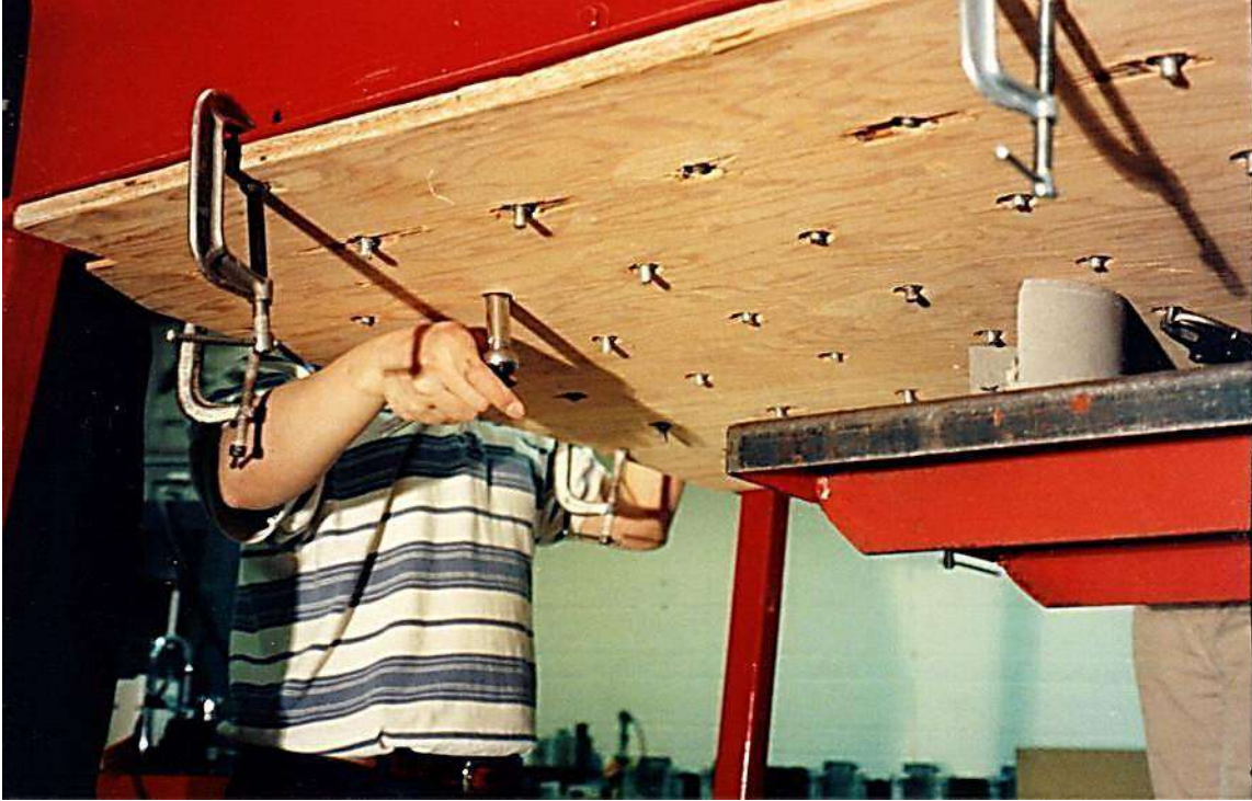
Figure 12: Holding the bottom nut during bolt tightening.
