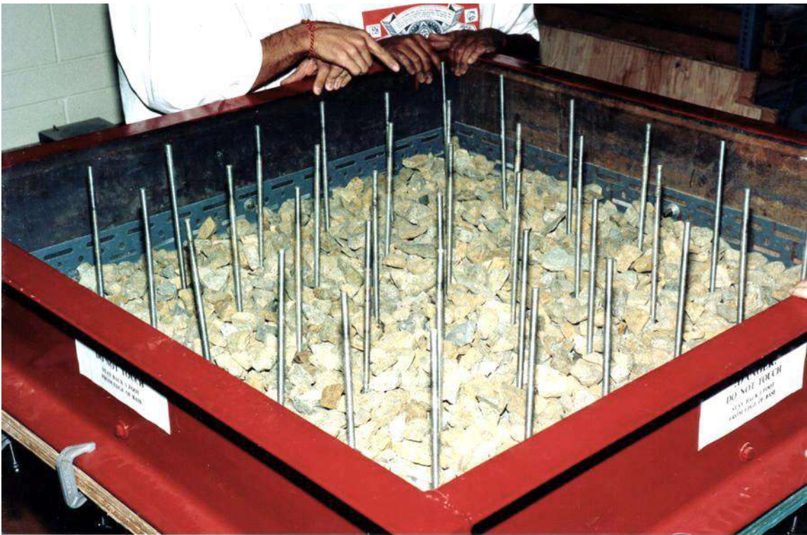
Figure 9: Placing the gravel in the frame.
