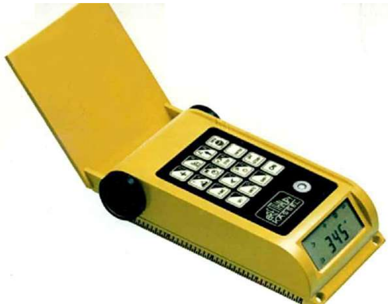
Figure 6: A Clar electronic geological compass manufactured by F.W. Breihapt in Germany.
