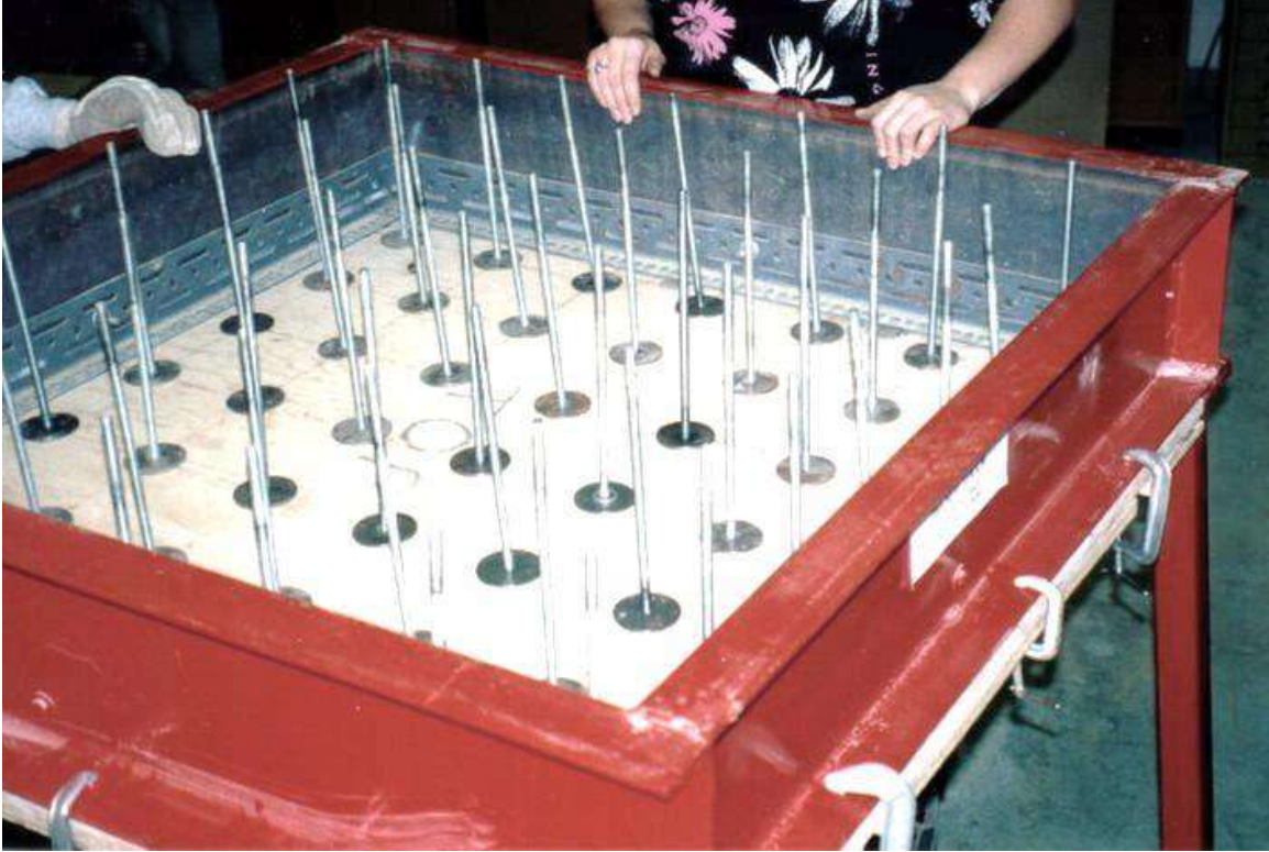
Figure 8: The rockbolts in position ready for the gravel to be placed.
