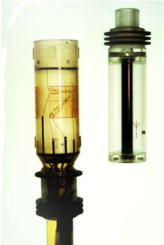
Figure 12: A cell for measuring the in situ triaxial stress field in a rock mass, developed in Australia (Worotnicki and Walton 1976). The hollow cylinder (on the left) is filled with adhesive which is extruded when the piston (on the right) is forced into the cylinder.
