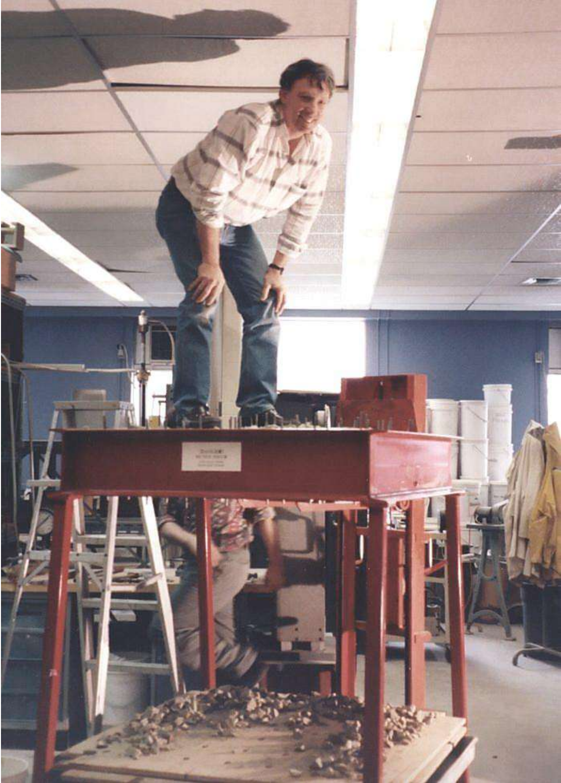
Figure 14: The load-carrying capacity of the bolted gravel plate.
