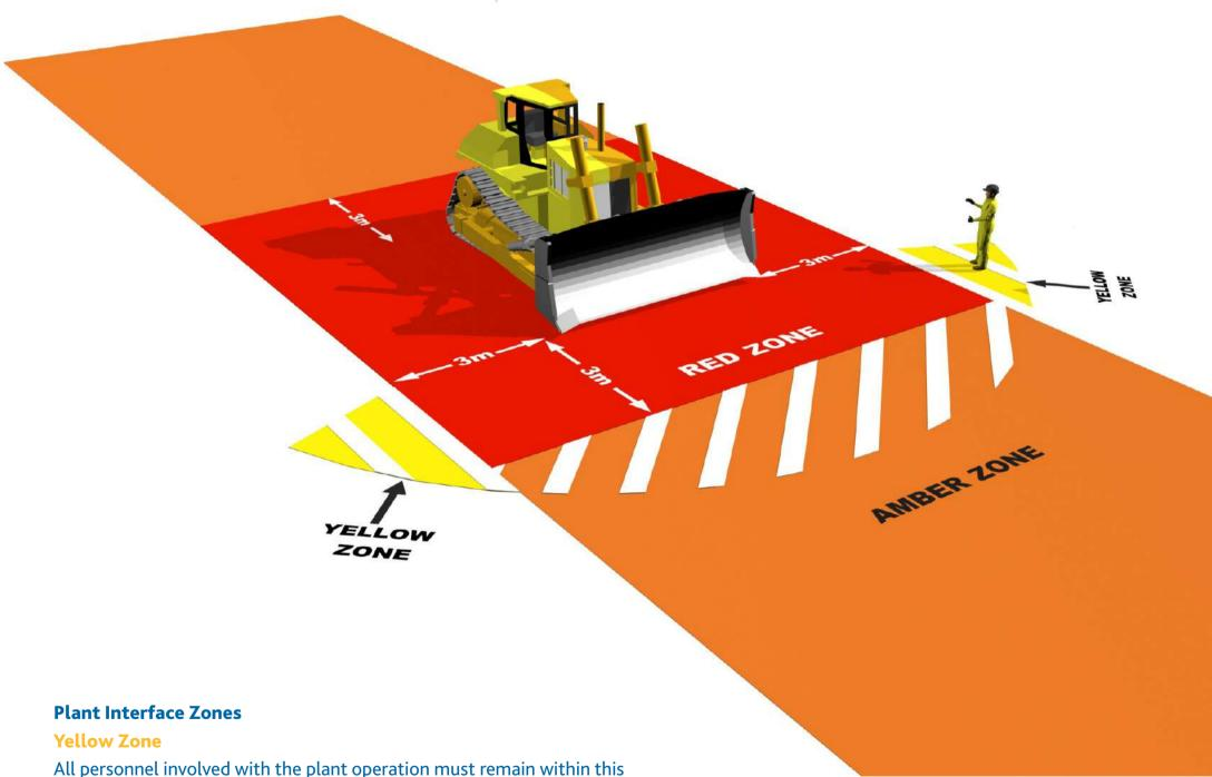
All personnel involved with the plant operation must remain within this zone to maintain visual contact with the plant operator.
