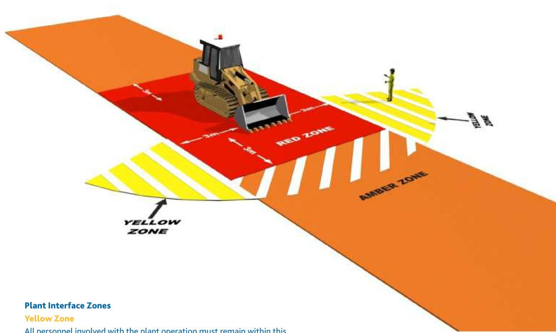
All personnel involved with the plant operation must remain within this zone to maintain visual contact with the plant operator.
