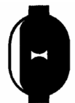
DRAG WEAR Metal has been removed by abrasion.
