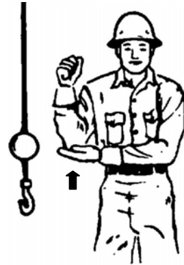
Fig. 4 USE WHIPLINE (Auxiliary Hoist). Tap elbow with one hand ; then use regular signals
