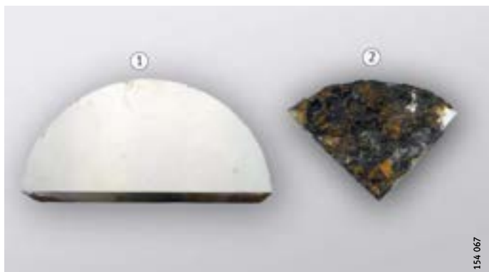
Figure 2 Corrosion resistance, comparison after 500 h salt spray test
