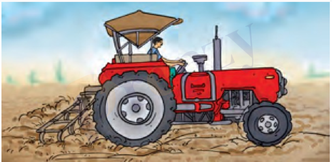
Fig. 1.1 (c) : Cultivator driven by a tractor
