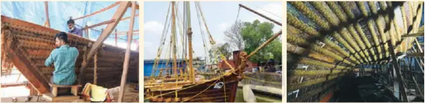
Fig. 7.9. Re-creation of a 5 th -century stitched ship
