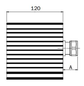
**006-100F:** Connector: 7/16" female, A=22mm **006-101M:** Connector: 7/16" male, A=31mm
