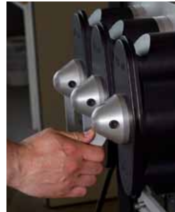
3. Continue to pull the lever upwards. This movement will affect the interlocking for a safe operation.
