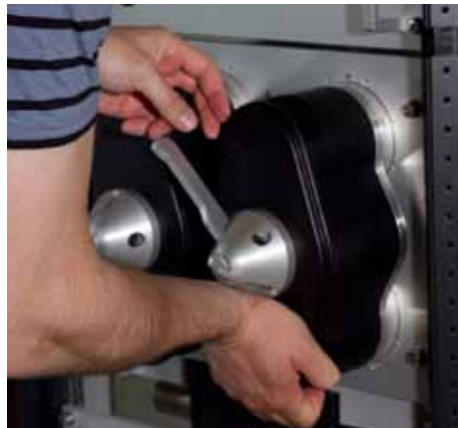
5. Turn the lever 45 degrees to the left and grab the U-link. The U-link is now released and ready to be removed.
