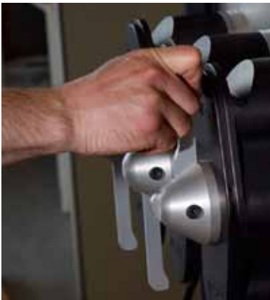
4. Continue until the lever is pointing straight up. The U-link is still fixed but the contact pressure is released.
