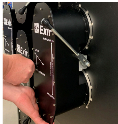
5. Pull the left handle downwards and hold firmly in the U-link. The U-link is now released and ready to be removed.
