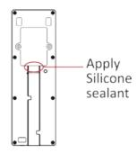
Figure 3-4 Apply Silicone Sealant
