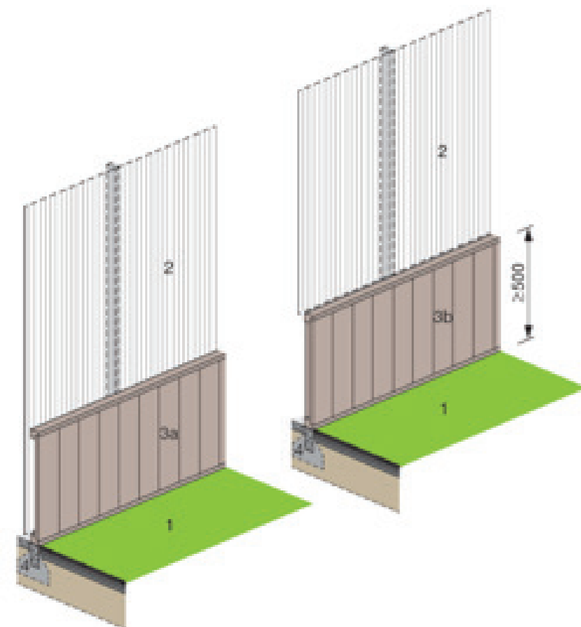
Figure 11 – perimeter fencing with containment panels used when the synthetic turf surface is laid up to the perimeter of the field
