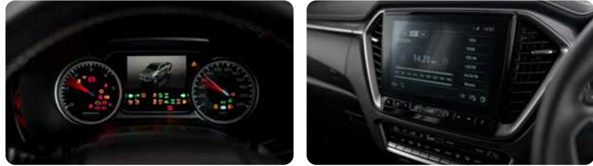
The display cluster is also linked to the infotainment system to reduce eye movement during driving and features second-row seatbelt reminders, allowing safety checks without the driver turning around.
