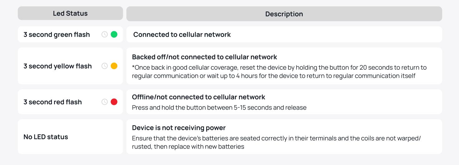
**NOTE:** To turn on the device, press the button for 5-15 seconds until the LED light turns green. To turn off the device, press the button for 5-15 seconds until the LED light turns red.
