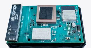
**A.** The device may be shipped in airplane mode. Open the case using a coin or flathead screwdriver to access the button, which can be found near the middle bottom of the circuit board.
