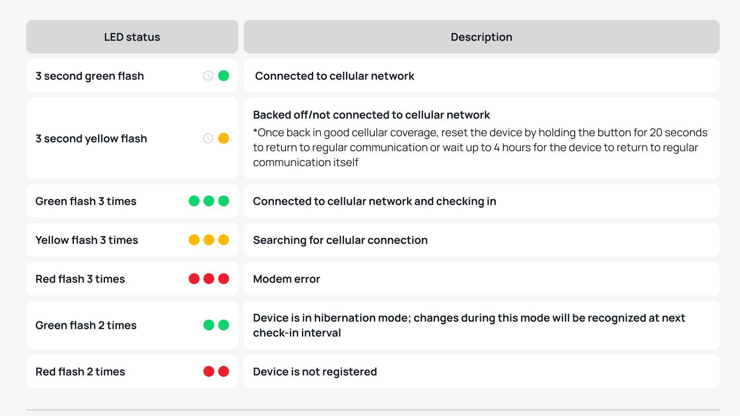
**NOTE:** To change the status from online to offline, press the button for 5-15 seconds and verify that the lights flash green to yellow to red. To reverse, do the same, but verify that the lights flash red to yellow to green, pause for 10 seconds, then flash from green to red to green.
