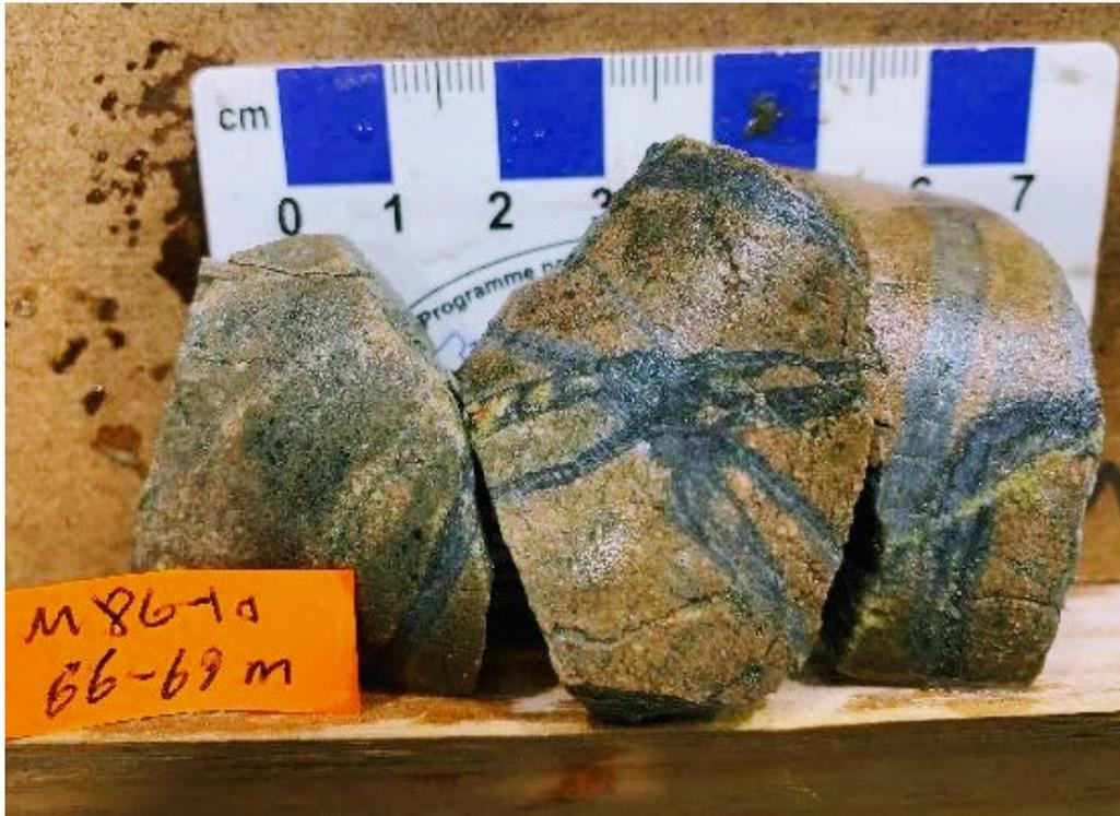
**Figure 3** – BK86-10 from 66.0-66.07 m. Strong potassic altered dacite with multi-generational quartz/quartz carbonate and epidote veining.
