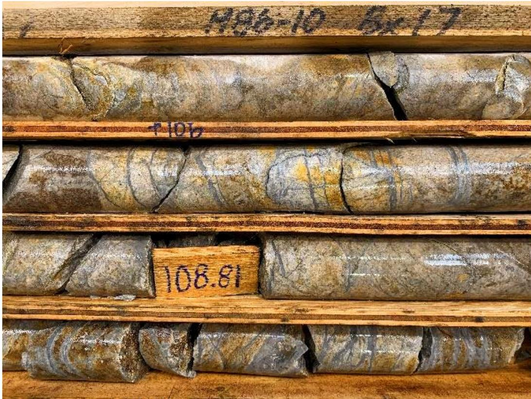
**Figure 2** – BK86-10 from approximately 105 m – 109 m (field of view). Altered dacite hosting multi-generational quartz/carbonate veining with pyrite/chalcopyrite.
