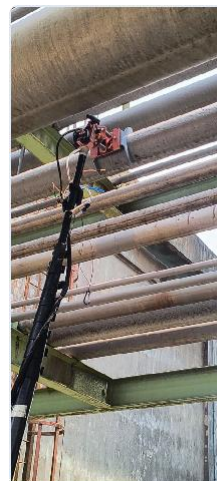
Figure 4: Curvature adapter enhancing probe stability and measurement accuracy on curved pipe surfaces
