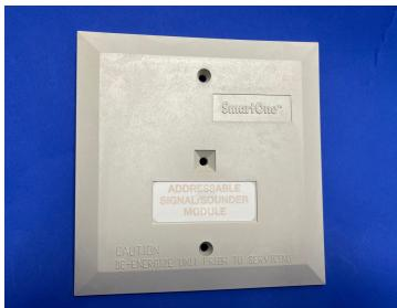
The SmartOne Addressable Signal Module (ASM), P/N 70-200200-003, is a notification appliance circuit that connects to the Signaling Line Circuit of a compatible control unit. The ASM is an intelligent field device that contains its own microprocessor, memory and the necessary electronics
