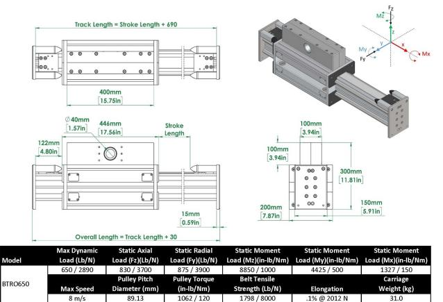
Please Note - the numbers in these drawings and tables represent performance parameters for our standard model. We can always customize a model more specifically to your application. Actual performance will vary pending motor/gearing selection.
