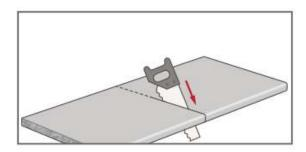
The best results will be achieved by cutting the worktop with a tolerance of +5mm, using a portable power saw (with the decorative side face down) or with a hand saw (decorative side face up). To finish the edge, use a portable hand router, straight edge and 'G' clamps. Clamp the straight edge to the worktop and ensure the cutter enters at the post-formed edge which will result in a perfectly straight, chip-free cut.
