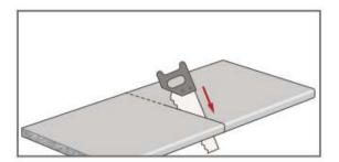
The best results will be achieved by cutting the worktop with a tolerance of +5mm, using a portable power saw (with the decorative side face down) or with a hand saw (decorative side face up). To finish the edge, use a portable hand router, straight edge and 'G' clamps. Clamp the straight edge to the worktop and ensure the cutter enters at the post-formed edge which will result in a perfectly straight, chip-free cut.
