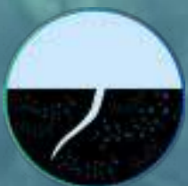
CAPILLARIES AND CRACKS WHERE MOISTURE ENTERS
