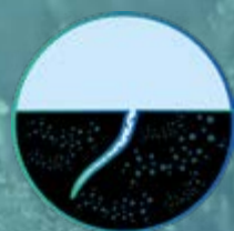
CRYSTALLIZATION CONTINUES UNTIL CRACKS AND CAPILLARIES ARE COMPLETELY SEALED
