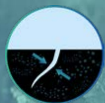
CONTACT WITH WATER INITIATES THE CRYSTALLIZATION PROCESS
