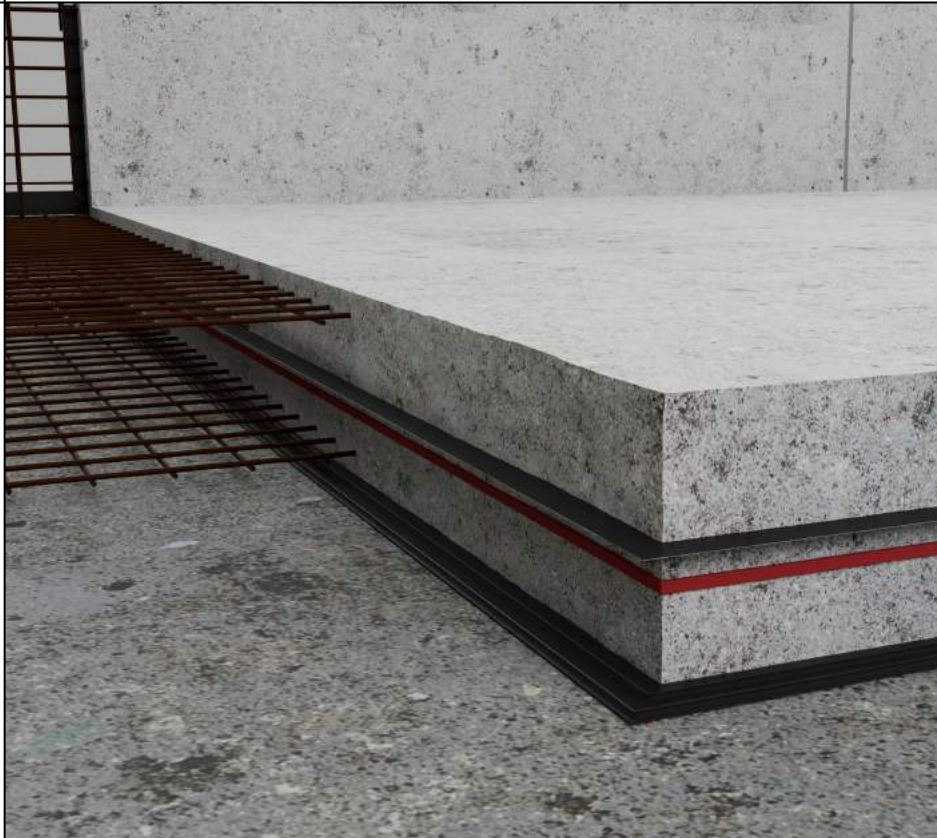
CASTING RESUMPTION JOINT BETWEEN TWO RAFT SLABS
