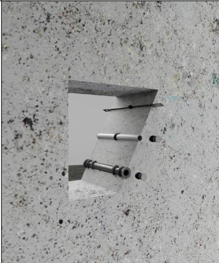
FORMWORK SPACERS WATERPROOFING
