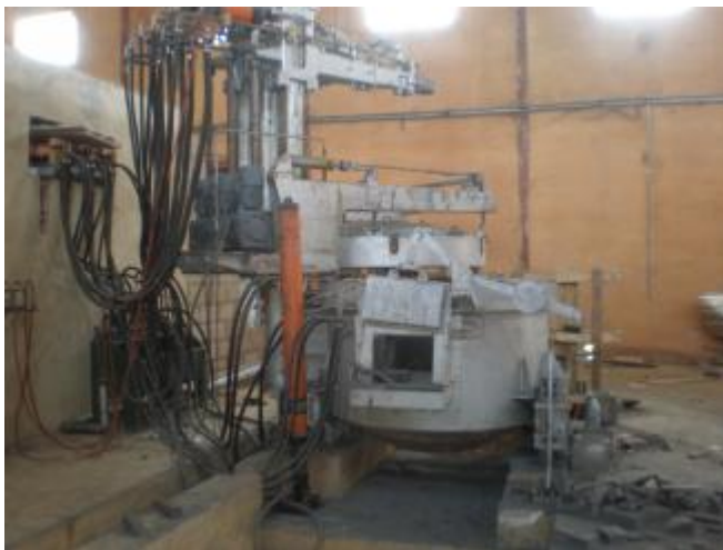
a) Electric arc furnace (NMDC, 2011)
