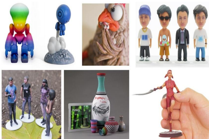
Fig.5.6 Objects printed using triple-jetting technology (PolyJet)
