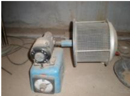
Fig. 4.13 Mouldability Index Tester
