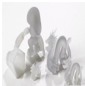
Fig.5.5 Objects printed using multijet printers
