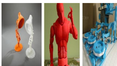
Fig. 5.4 Some objects printed using SLS Technology
