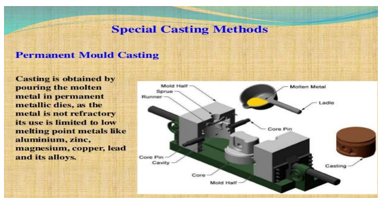
Fig.8.27 Permanent mould casting Illustrated
