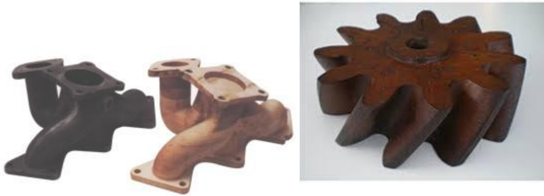
Fig.8.20 Some patterns used in producing auto-parts
