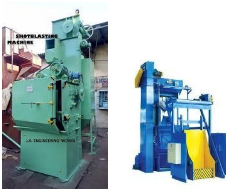
Fig.11.1 Two different makes of shotblasting machine (manufacturingmachines.com, 2020)
