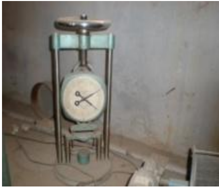
Fig.4.7 Spring Loaded Green Compression Strength Testing Machine
