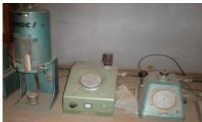
Fig.4.10 Manual and Electric permimeters
