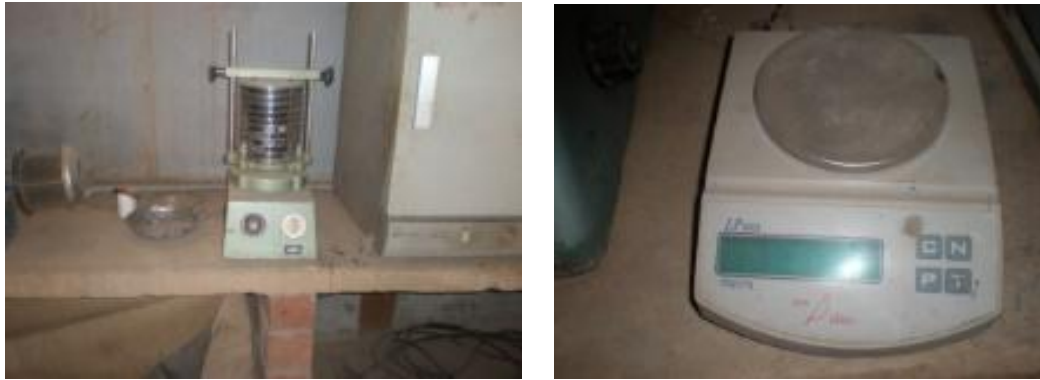
Fig. 4.15 Nest of Sieves mounted on a Sieve-Shaker and Digital Weighing Balance used for Weighing Retained Sand on Sieves
