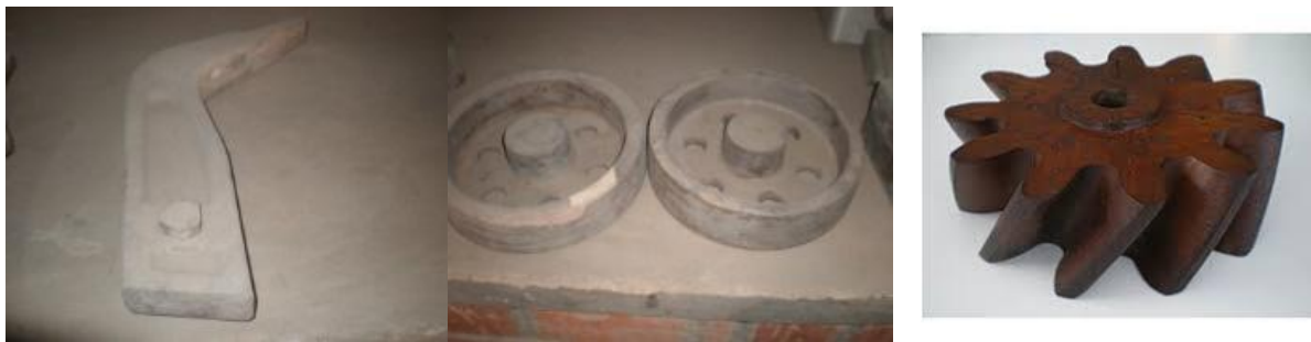
Fig. 4.20 Patterns used for making some Automotive Parts
