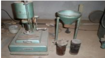
Fig. 4.6 Standard Rammer, pouring hopper and specimen tube for standard Specimen Preparation
