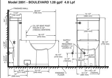
IMPORTANT: Water supply on the wall is required at 3-3/4" or 9" from centerline of the toilet (see rough-in). First suggested position is hidden behind the toilet. The geometry of the toilet gives space for this installation. The second suggested position is next to the toilet. Between these two positions, the space for the supply between wall and toilet is limited to 3-1/4". In this case, check your supply and hose dimensions.
