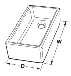
**D:** 17-7/8" TO 18-3/8" (454 TO 466 mm) W: 29-3/4" TO 30-1/4" (756 TO 768 mm)
