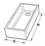
D: 17-7/8" TO 18-3/8" (454 TO 466 mm) W: 35-3/4" TO 36-1/4" (908 TO 920 mm)
