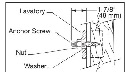
2. Apply a bead of silicon to the back of the lavatory. See Diagram.
