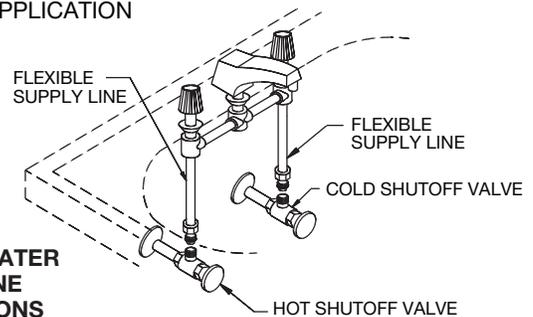
**TYPICAL WATER SUPPLY LINE CONNECTIONS**
