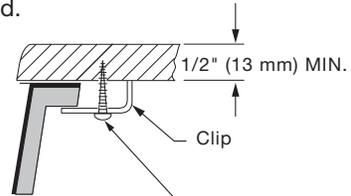
Drill 1/8" (3 mm) dia. X 3/8" (10mm) deep #10 Wood Screw
