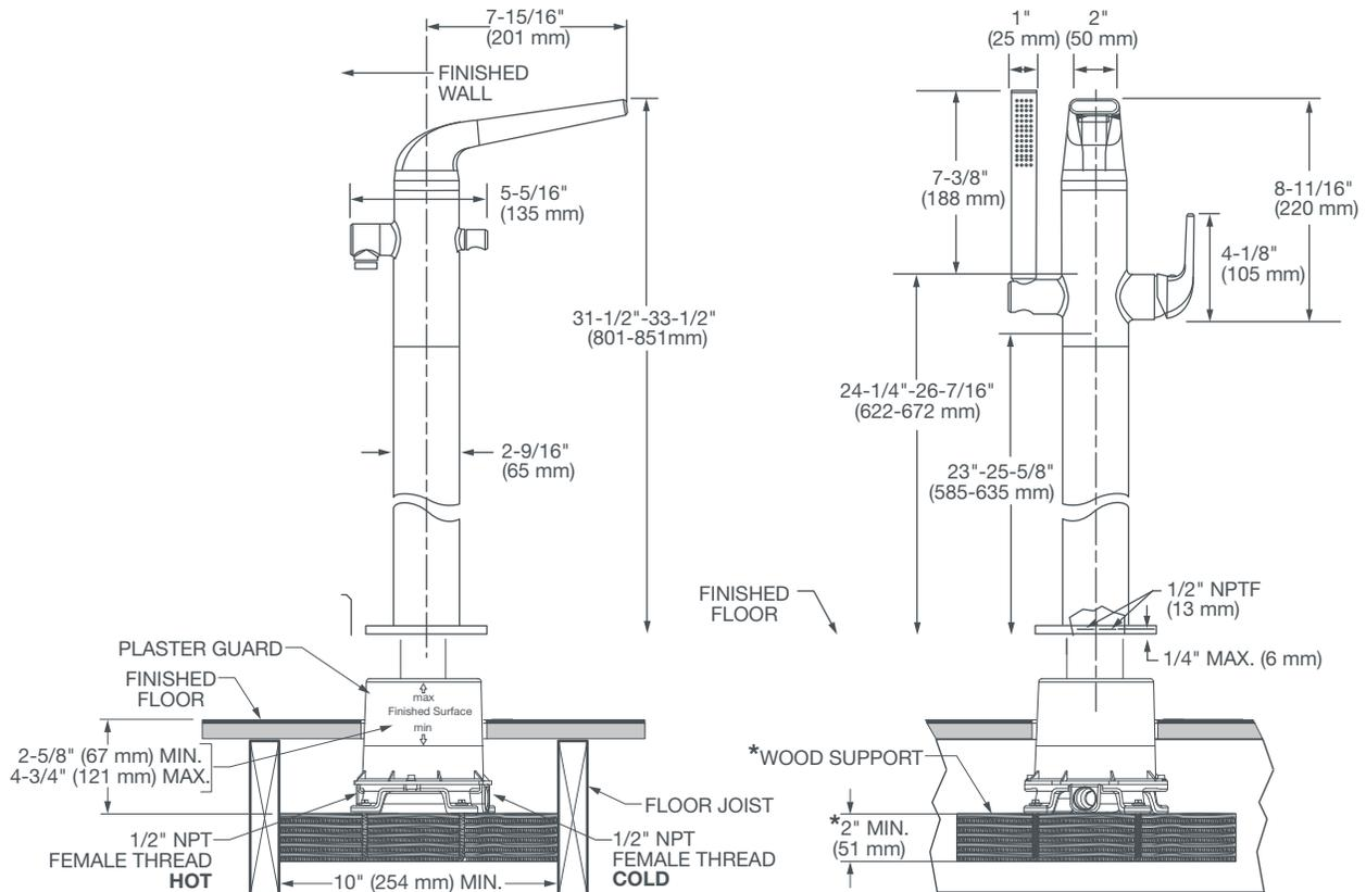
**\*Adequate floor support is required. The wood support must be a minimum of 2" (51 mm) thick by 10" (254 mm) wide. 2x6 lumber is NOT adequate for this application.**
