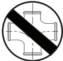
Depending upon your plumbing and venting conditions, the flow from the toilet in a back-to-back installation may create a vacuum on the system and draw water from the opposing bowl. The National Standards Plumbing Code prohibits the use of a cross fitting for drainage as throw over is possible. The code does approve a directional "Y" style fitting with proper venting to direct the water downward and away from the other toilet.
