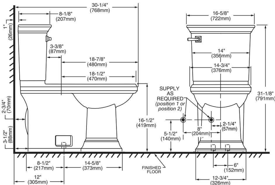
**IMPORTANT:** Water supply on the wall is required at 2-1/4" or 8" from centerline of the toilet (see rough-in). First suggested position is hidden behind the toilet. The geometry of the toilet gives space for this installation. The second suggested position is next to the toilet. Between these two positions, the space for the supply between wall and toilet is limited to 3-1/2". In this case, check your supply and hose dimensions.
