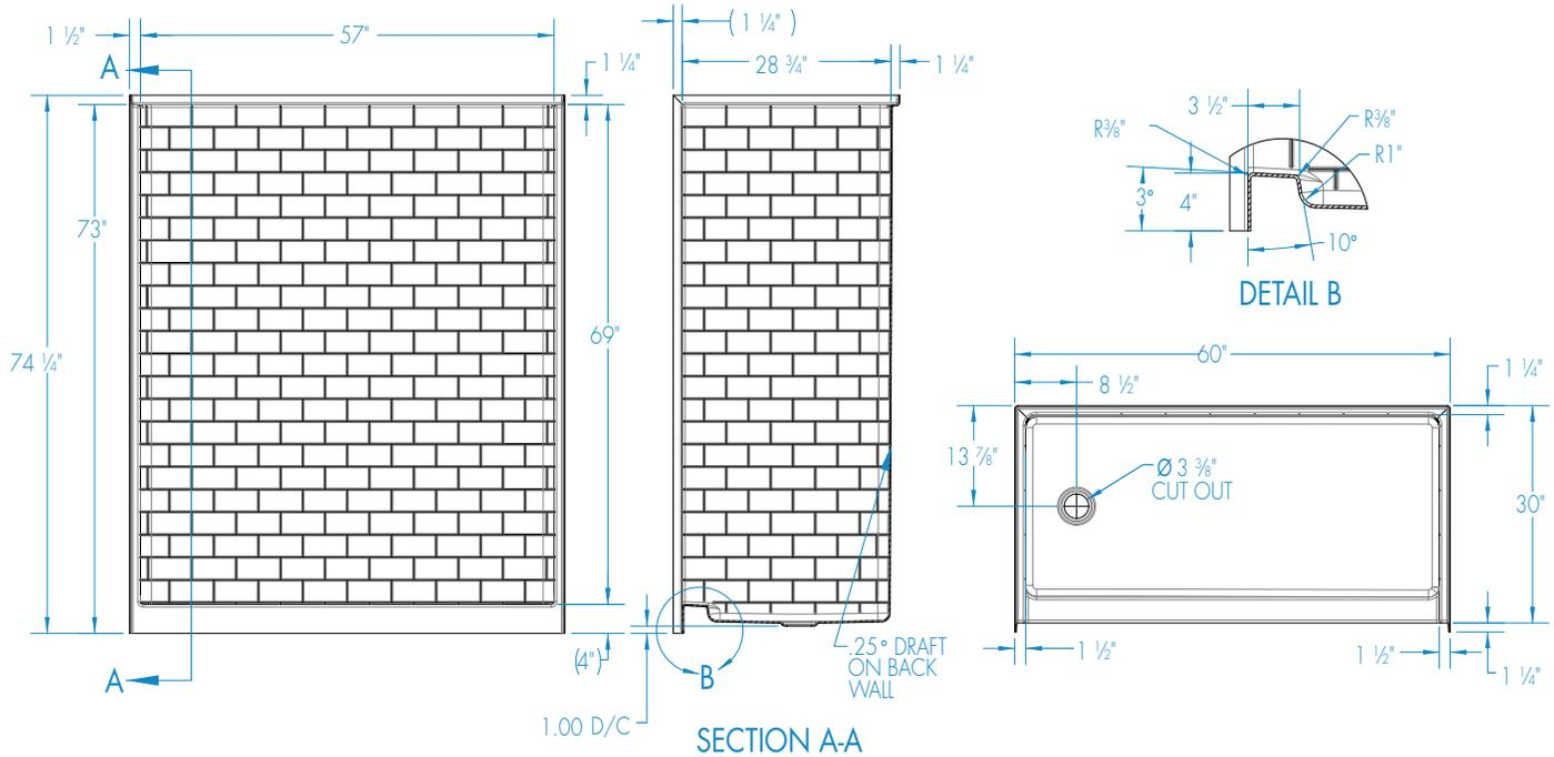
**FEATURES** Dimensional Tolerance  $\pm \frac{3}{8}$ ". Dimensions needed for site preparation should be measured from the unit. Aquatic assumes no responsibility for preparatory work.
